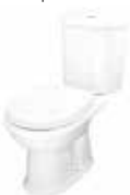
Closed Coupled Toilet Suite 4822902 S-Trap , WELS 4 Star, 4.5L/Full, 3L/ Half, 3.4L/Avg Flush, L05505
